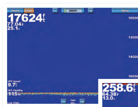
The images show the fantastic target separation and depth capabilities of Spread Spectrum Chirp technology. To be able to reach depths more than 5 000 meters at a boat speed close to 10 knots says something about this great technology and the GSD 26 from Garmin.
